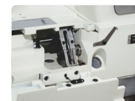
打线凸轮外移 The threading cam moves outwards
