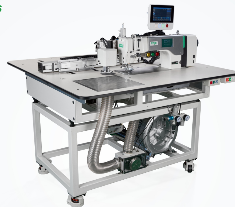
小范围、台面吸风、带振动刀 Compact workspace, desktop suction, vibrating knife
