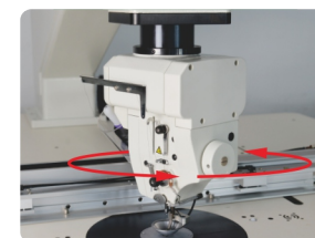
机头360°任意旋转 360° arbitrary rotation of the machine head
